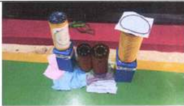
Pemasangan Primary Fuel Filter Genset CH10930
